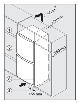
\* The appliance depth is increased by approx. 35 mm for appliances with wall spacers fitted.
